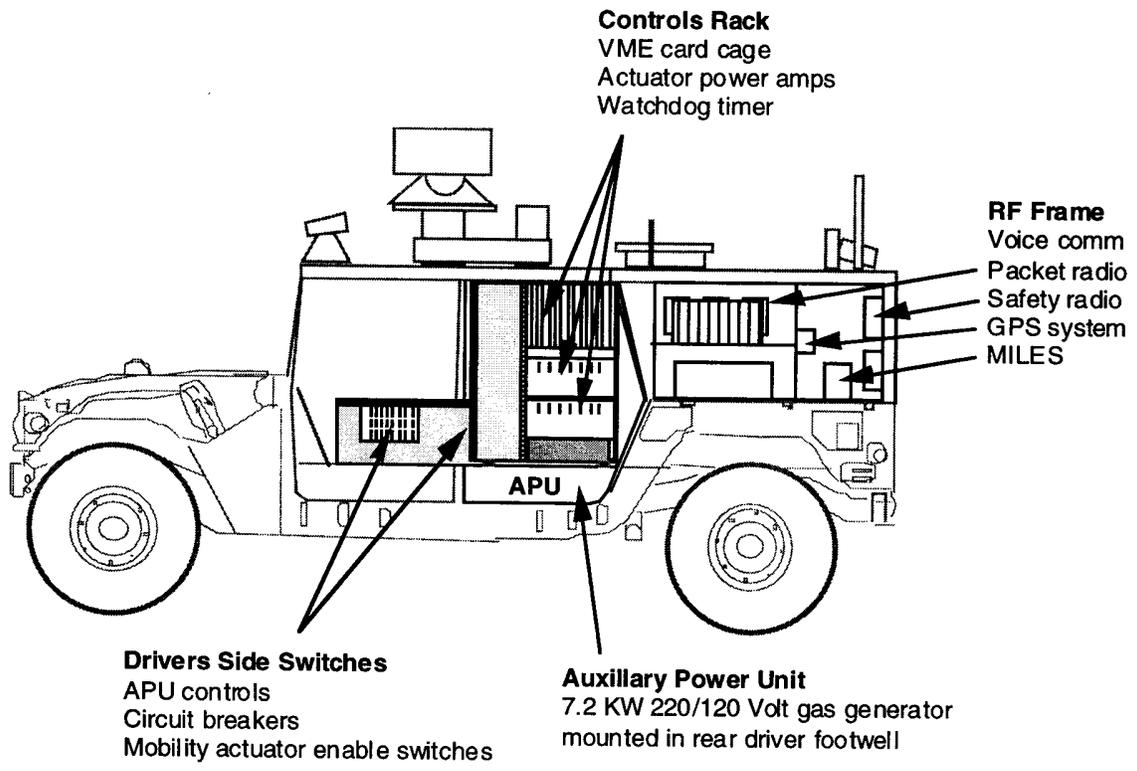
Figure 7. Driver's side view of SSV equipment.
