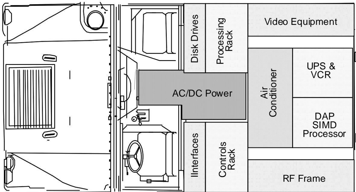
Figure 5. Configuration of equipment areas inside SSV-B, C and D.
