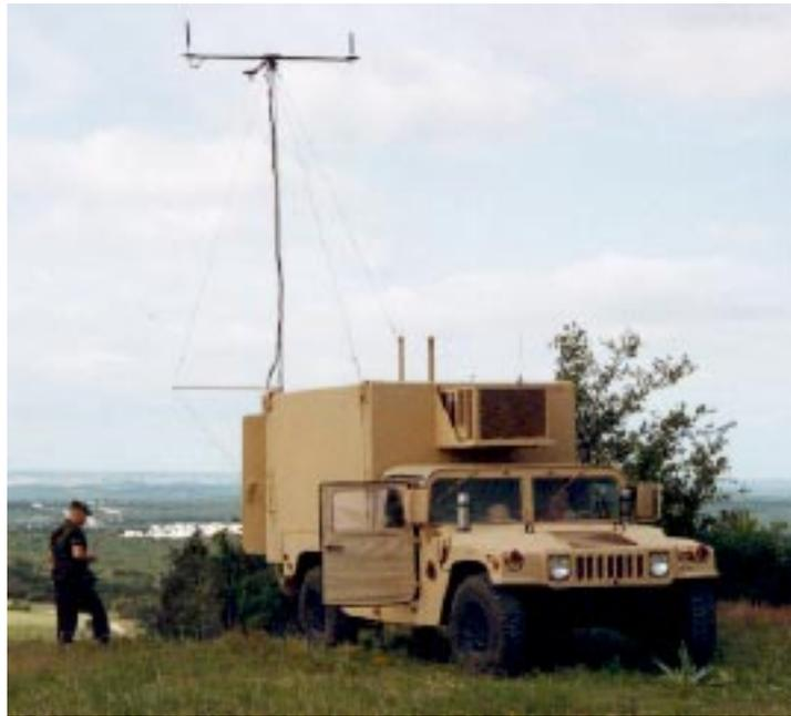
Figure 4. BASE vehicle, which contains the multi-vehicle operator workstation.
