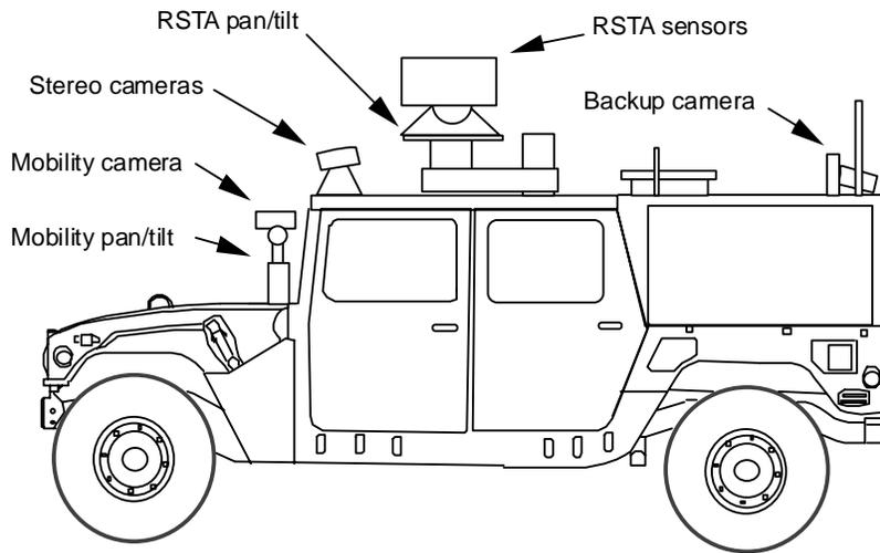
Figure 8. Placement of mobility and RSTA sensors on the SSV.
