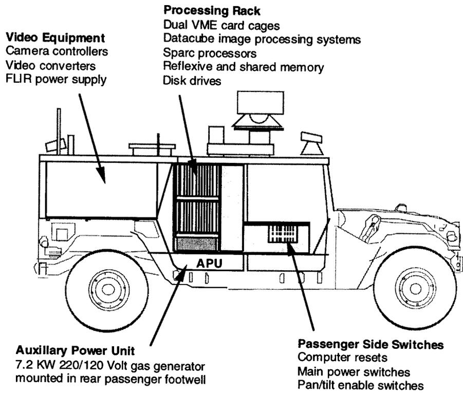
Figure 6. Passenger's side view of SSV equipment.
