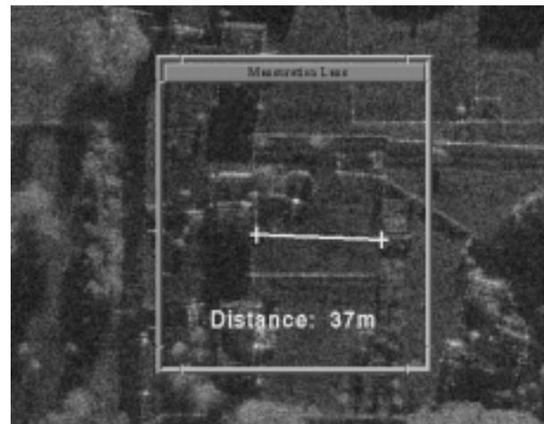
FIGURE 7. This mensuration lens shows the length of a line segment manipulated by dragging the line's endpoints through the lens.
