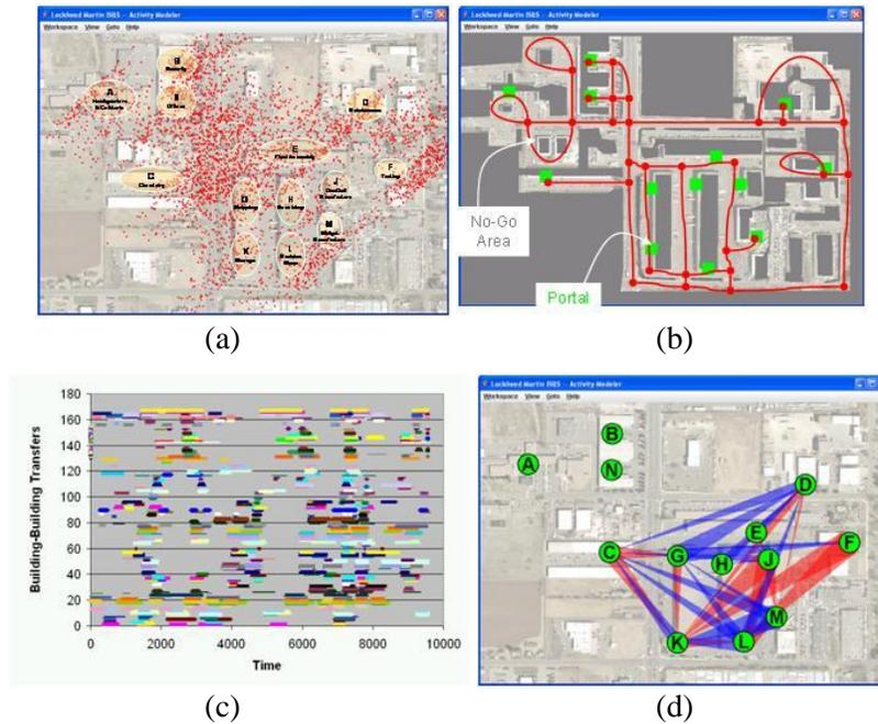
Figure 1-11. (a) Short tracks are constructed from these raw GMTI dots (simulated data). (b) “no-go” graph used to constrain interpretation of low quality tracks. (c) Individual transits detected between buildings. (d) Links in network derived from repeated transits.
