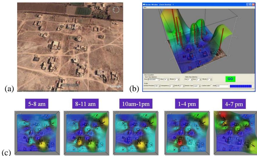
Figure 1-2. (a) Area covered by sensor network. (b) Visualization tool for creating 3D heatmaps. (c) Example showing spatial structure of activity during several time intervals.
