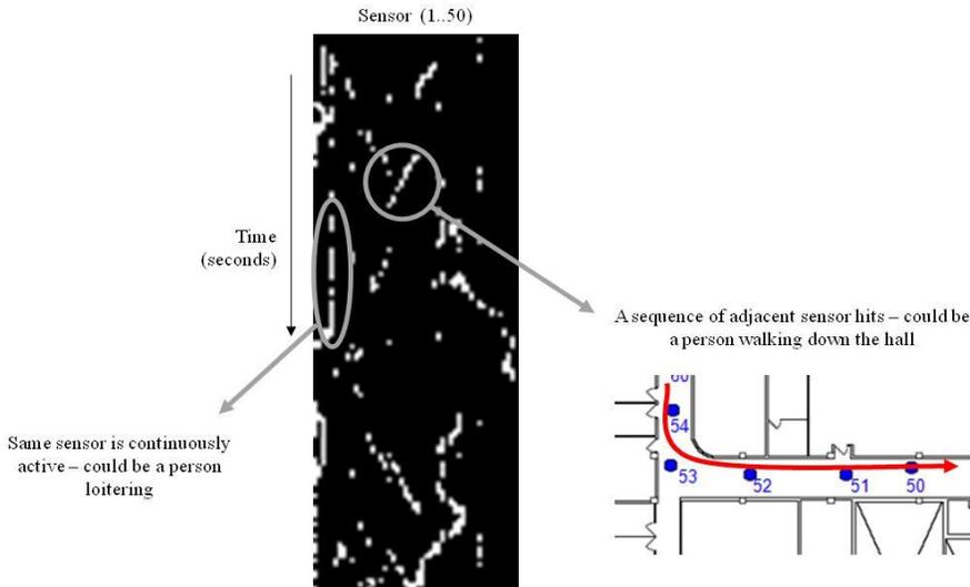
Figure 1-9. Example of sensor network data in the form of a two dimensional matrix.
