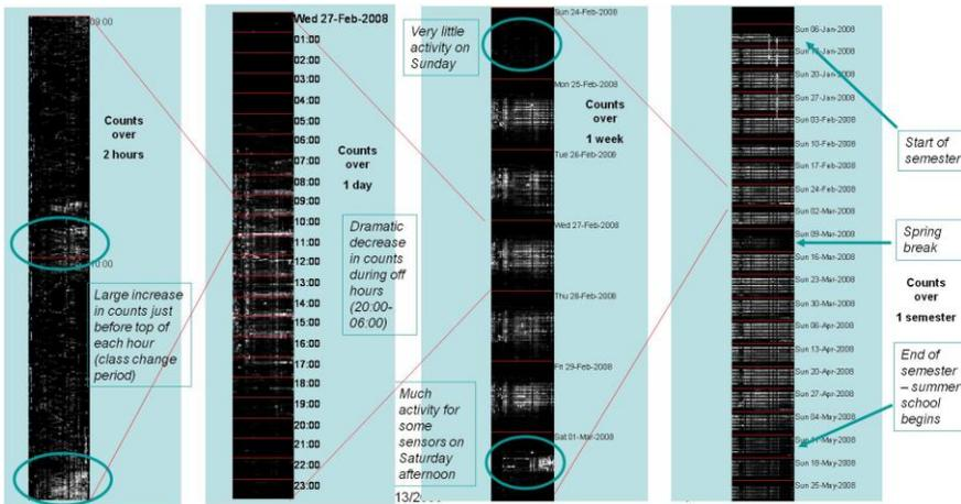
Figure 1-4. Visualization showing temporal structure of activity in a building. Rows are time steps. Each tiny column is one node in a network of passive infrared motion detectors.
